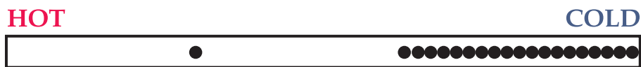
Figure 1.7: The horizontal array of inelastic particles of Chapter 5: A single particle commutes between the hot left side and an almost immobile cluster at the right.
